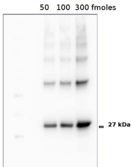
Following standard western blot procedure this image was obtained using a CCD imager (FluorSMax, Bio-Rad) and Quantity One software (Bio-Rad) as described below. Note: Optimal quantitation is achieved using moderate sample loads per gel lane, generally 0.5 to 2.5 ug total protein, depending on the abundance of the target protein.
